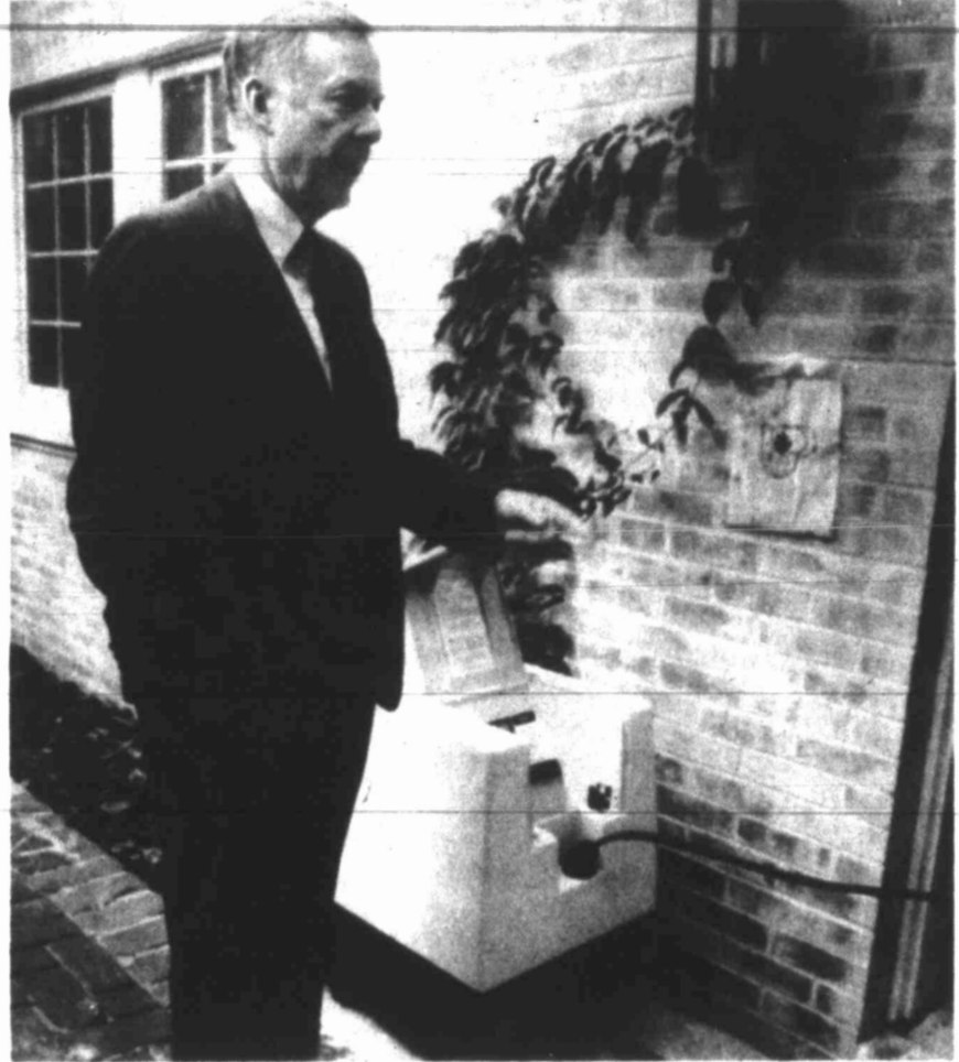
UNIVERSITY PARK — T. Boone Pickens displays a fueling station at his home in a Dallas suburb Thursday morning. The device compresses natural gas and injects it into the storage canister of an automobile that is powered by the gas. Costs to make the conversion and obtain the compressor total about $5,000.
