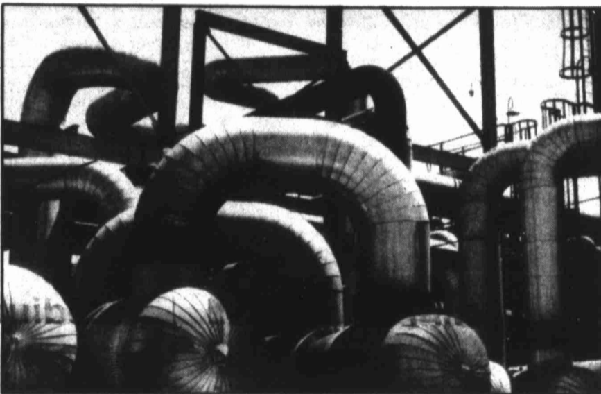
A convoluted mass of tubing serves as an energy-conserving heat exchanger for crude oil refining at the Big Spring Fina Oil and Chemical Co. refinery. The system takes waste heat from refined products leaving a unit and heats incoming raw material, thereby saving on heating costs.
