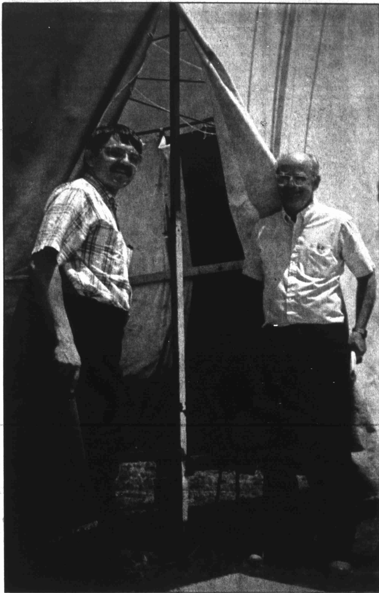
Soil scientist Dr. Ted Zobeck, left, and research leader Bill Fryrear stand in front of a rainfall simulator at the Agricultural Research Center. The simulator helps the scientists study the effects of rainfall by using different water pressures on different soils to determine the rate of change in soil properties due to rainfall.
