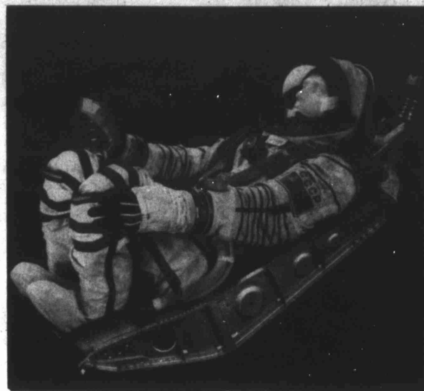
Kazbek "space couch," special seating in each Soyuz capsule in which cosmonauts are launched and returned to earth. The seats are designed to help cosmonauts withstand the "g-forces" experienced during re-entry.
