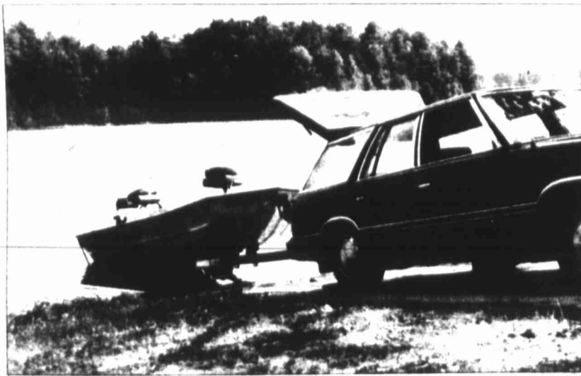
"DUNKING" TRAILER—Trailer wheel bearings can be adversely affected by "dunking" trailers during the launch of boats. Bearings may need to be repacked afterwards.
