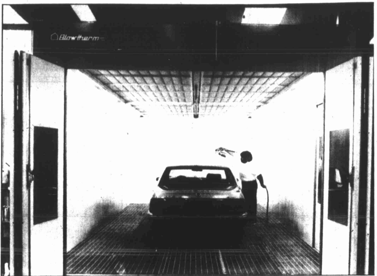
The new Blowtherm Ultra spraybooth oven produces the finest finish on automobiles this side of the factory. The facilities at Pat Gray Body Works underwent extensive alterations to accommodate the imported equipment. A factory-perfect paint job is made possible by perfectly controlled air, humidity and temperature. The Blowtherm Ultra is exclusive at Pat Gray Body Works, located at 700 N. Owens. Drop by and take a look.
