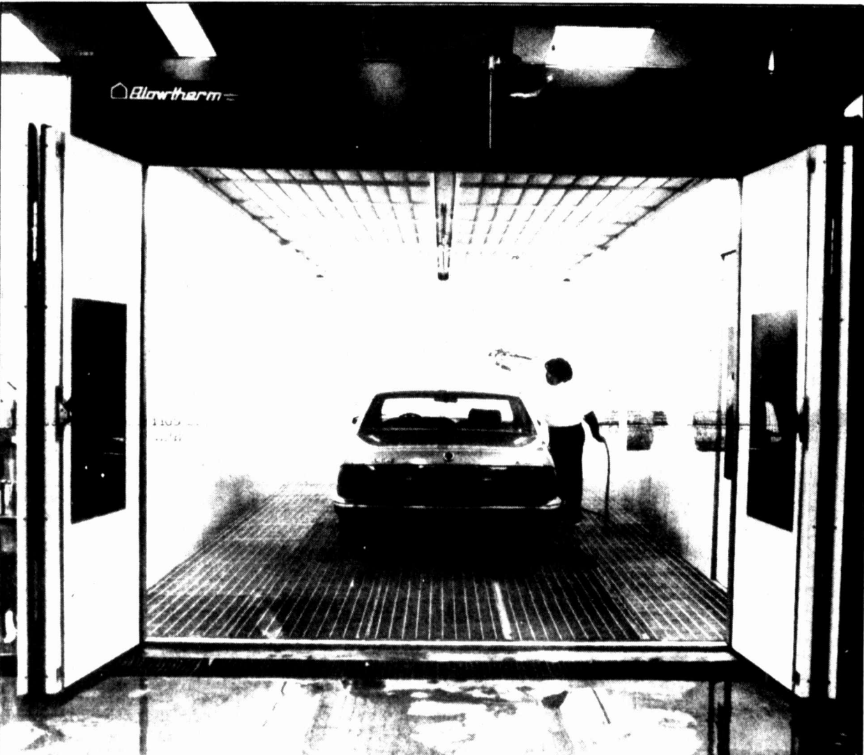
The new Blowtherm Ultra spraybooth oven produces the finest finish on automobiles this side of the factory. The facilities at Pat Gray Body Works underwent extensive alterations to accommodate the imported equipment. A factory-perfect paint job is made possible by perfectly controlled air, humidity and temperature. The Blowtherm Ultra is exclusive at Pat Gray Body Works, located at 700 N. Owens. Drop by and take a look.
