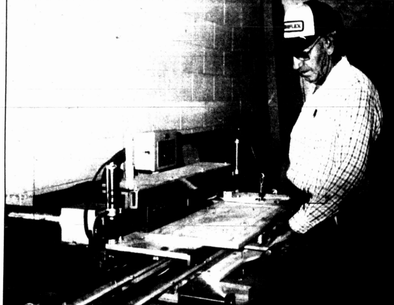
Denver Harris demonstrates his mastery of a raised-panel door machine used in the construction of custom cabinetry. He and son, Gary, build fine hardwood products — including furniture — at Harris Cabinet Works, 2810 FM 700.
