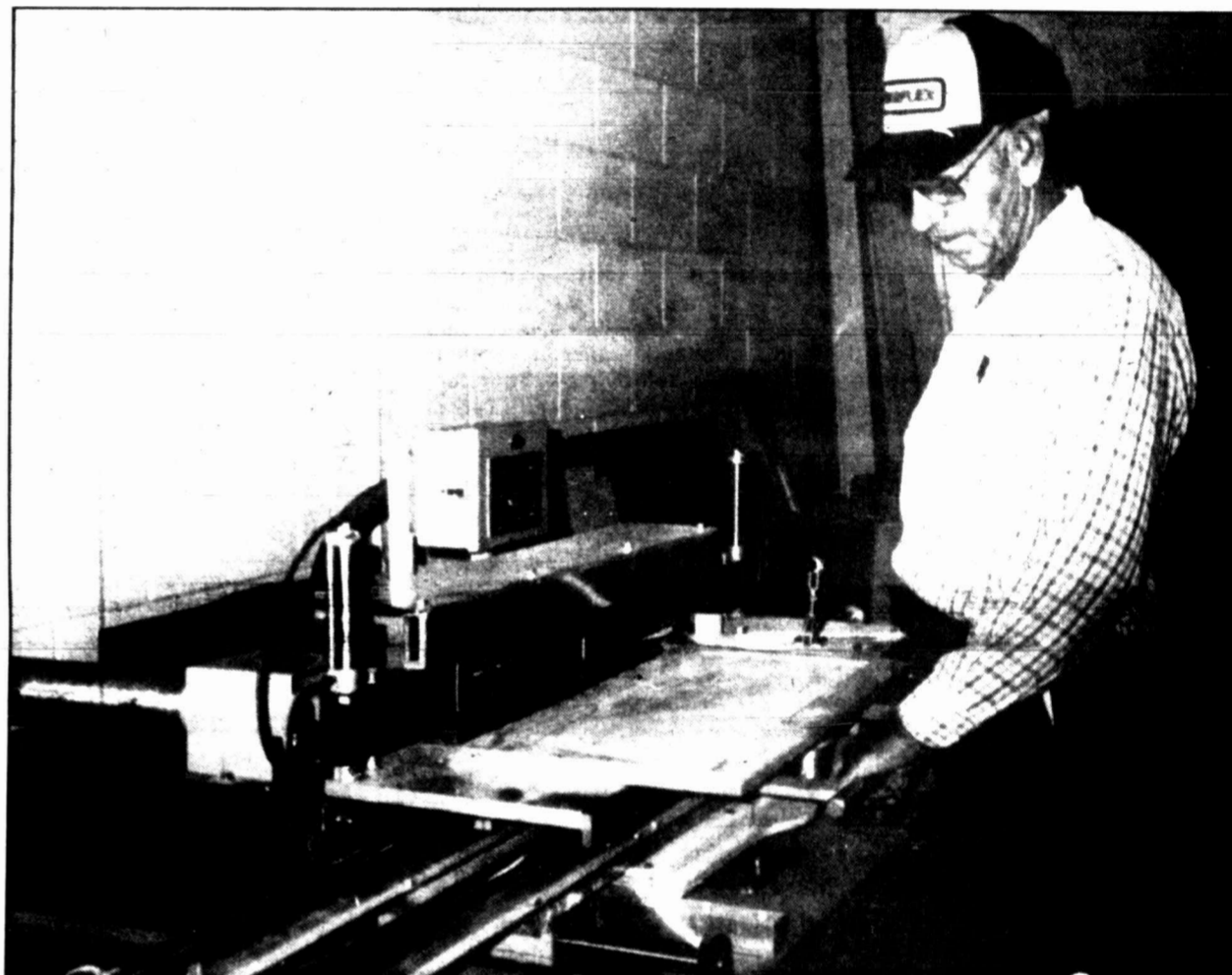
Denver Harris demonstrates his mastery of a raised-panel door machine used in the construction of custom cabinetry. He
