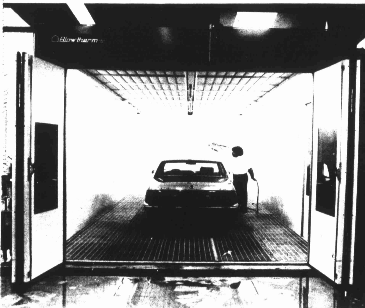
The new Blowtherm Ultra spraybooth oven produces the finest finish on automobiles this side of the factory. The facilities at Pat Gray Body Works underwent extensive alterations to accommodate the imported equipment. A factory-perfect paint job is made possible by perfectly controlled air, humidity and temperature.
