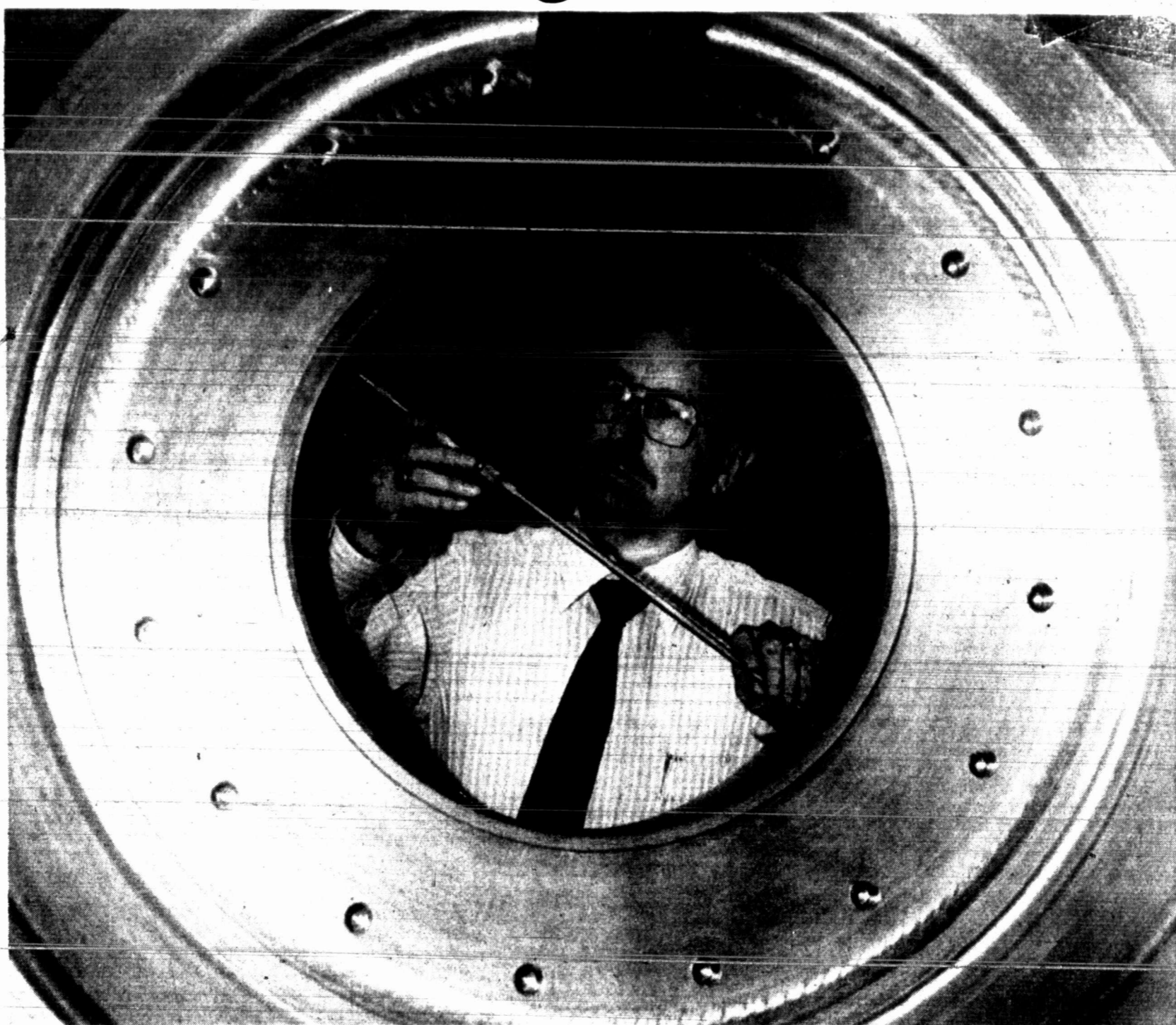
Bob Boyles of J&M Oilfield Supplies examines the inside diameter of a blow-out preventer body at the company's machine shop.
