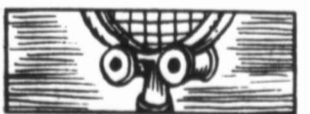
Tack a pair of spoons close together on a wall to make a broom or tennis-racket holder.
