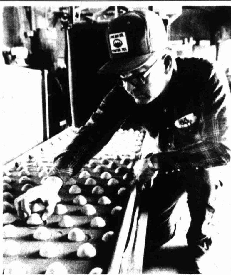
CONDUCTS DENSITY TEST Fryrear inspects simulated soil cots in test for wind erosion
