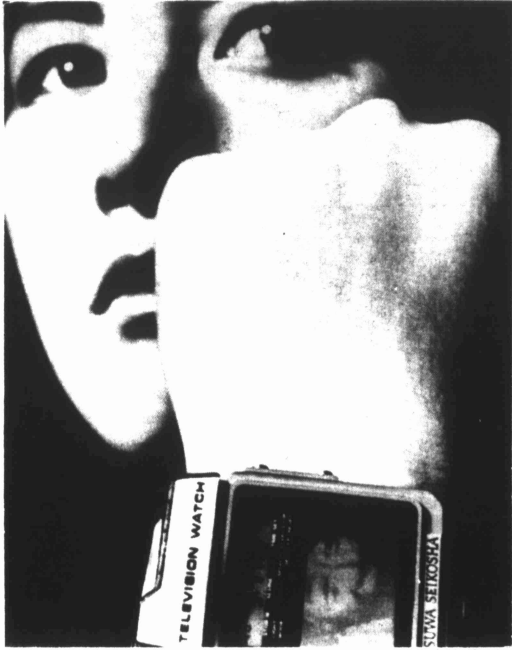
WATCH TV ON TV WATCH—Seiko announced in Tokyo Wednesday the world's first wrist-watch with a black-and-white television screen, featuring a 1.2-inch liquid crystal display. The watch is capable of receiving regular VHF, UHF and FM broadcasts and comes with a battery-powered wallet-size receiver and a headphone. Though the wrist TV is not yet on the market, it is expected some time next year for a selling price of around $400.
