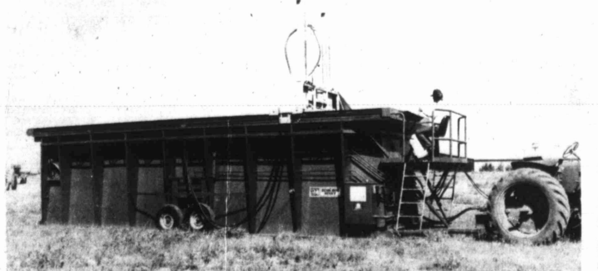
GIANT HELPER — The module builder has helped separate the ginning and harvesting operations so that growers can keep on harvesting even though the gin may be backlogged or down for repairs.
