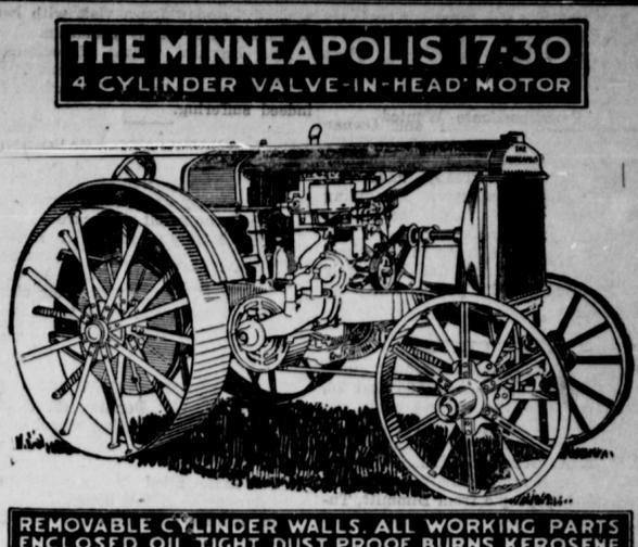
REMOVABLE CYLINDER WALLS. ALL WORKING PARTS ENCLOSED. OIL TIGHT, DUST PROOF, BURNS KEROSENE
