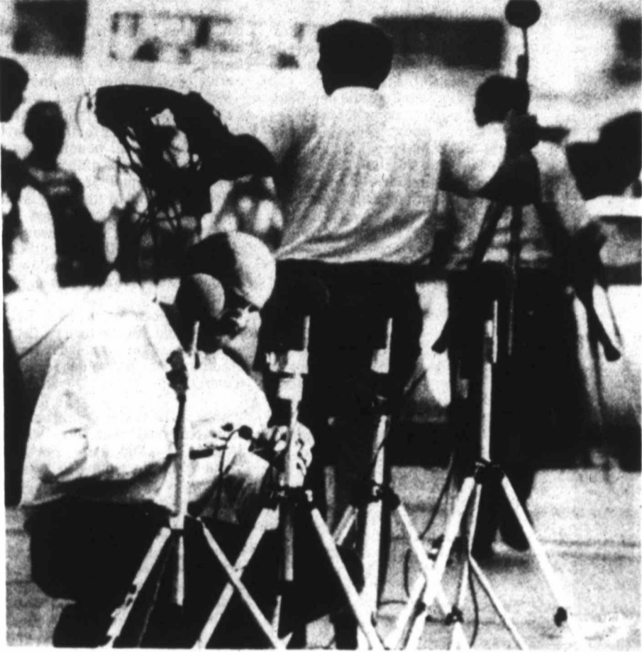
POSITIONING THE MICROPHONES — Sound experts from Bolt, Beranek and Newman adjust and position microphones around the President John F. Kennedy assassination site in Dallas Sunday. Rifle fire from police department sharpshooters was recorded and will be compared to a recording of the actual assassination. The Boston firm will try to determine how many shots were fired at President Kennedy on Nov. 22, 1963. The results will be given to the House Select Committee on Assassinations by Sept. 1.
