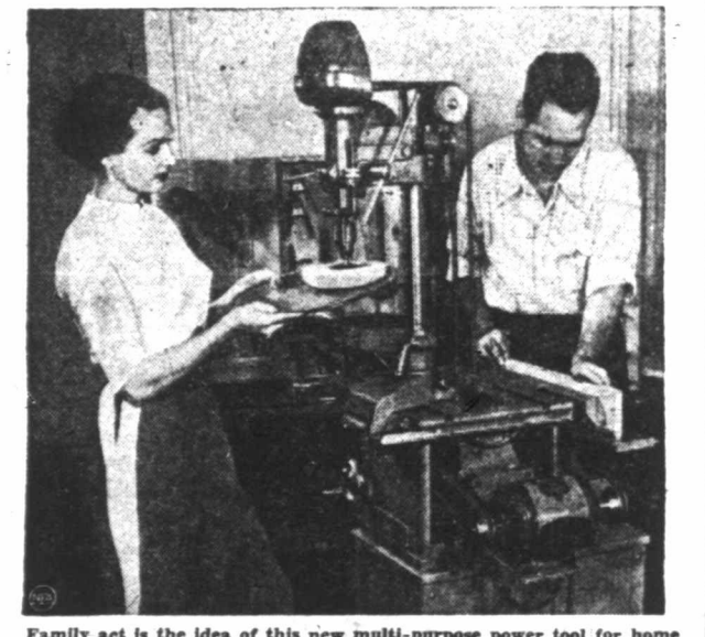
Family act is the idea of this new multi-purpose power tool for home workshops. While pop uses the jointer to build a cabinet, mom's using the drill press to shine the silver.
