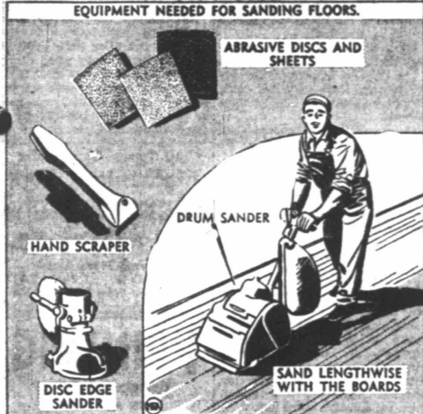
Power sanding will help you achieve the smooth surface essential in floor refinishing and takes less time than other methods.
