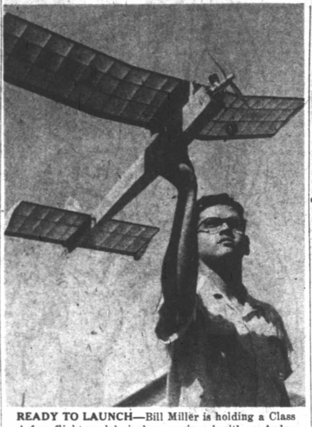
READY TO LAUNCH —Bill Miller is holding a Class A free flight model airplane equipped with an Arden engine. The miniature aircraft weighs 11 ounces and has a 42-inch wing span. Restricted for contests to a 15-second engine run, it is capable of motor-driven flight up to eight minutes on its fuel mixture of castor oil and alcohol.
