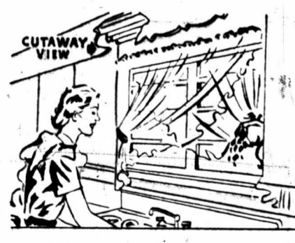
AT THE SINK: A lighting unit placed above the sink as illustrated keeps you from working in your shadow. You'll be able to easily see the dishes are clean—saving energy and disposition.
