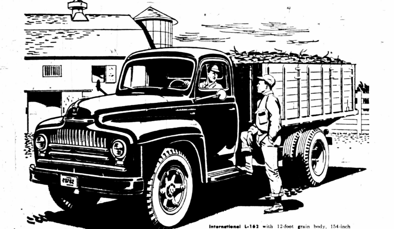
International L-162 with 12-foot grain body, 154-inch wheelbase, GVW 18,000 lbs. Has a bumper crop of special features to help you handle a wide variety of loads. Specifications subject to change without notice.
