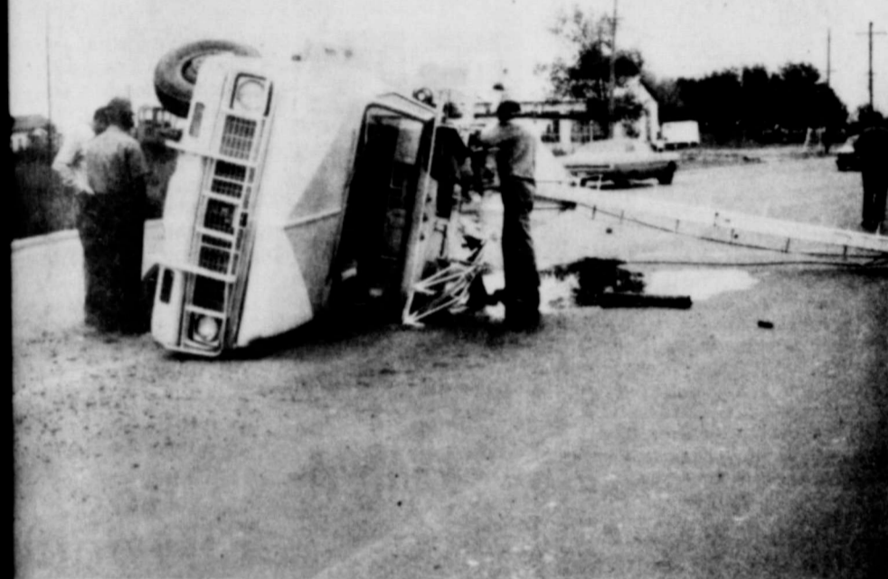
DAMAGE to this H & H Well Service truck, as well as to TV Cable and telephone lines occurred Tuesday morning. Jerry Holton, driver, was not injured. The hydraulic system evidently failed, causing the 20-foot tower mounted on the truck to lift, and when it did so, it gathered up TV cable and telephone lines, pulling the truck over its side according to chief of police, Leland Wood.
