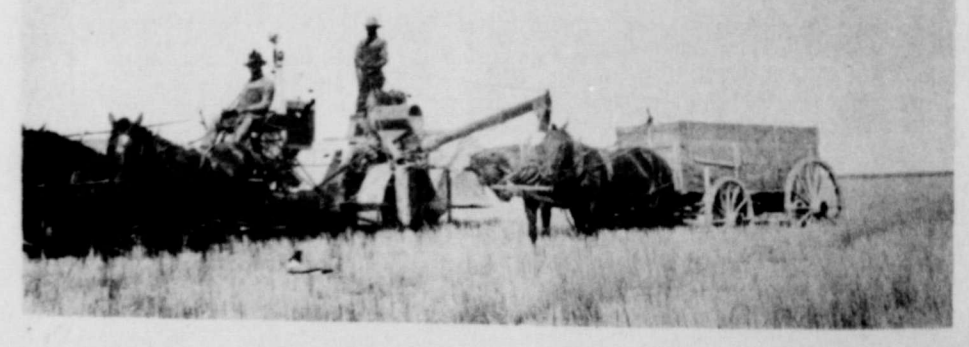
HARVEST 52 YEARS AGO: Combined Harvester and thresher of Paul Higgs - in field of Walter Wilmet. This was taken when machine was standing still - wagon was receiving grain - is standing still a little rear of spout which delivers grain when threshed. Picture shows height of stubble after being headed. Field is 25 bushes per acre.
