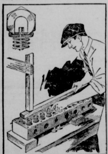
Using a Slotted Nut and a Wooden Lever to Compress Auto-Valve Springs.
