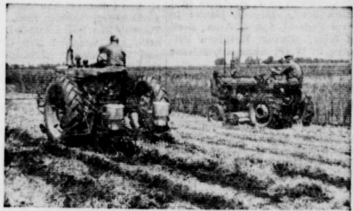
Hammer mower and mulch planter at work in a fall seeded ryegrass cover-crop. No plowing or cultivation.
