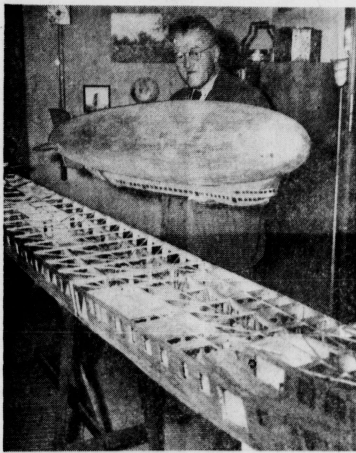
FOR THE FUTURE —German aviation engineer Albert Simon holds a model of a new airship he hopes to put into production. Below the model is a larger design of the dirigible's nacelle which will stretch for almost the entire length of the craft. Unlike the zeppelin of former times, Simon has planned his new one to take off from—and land on—water.
