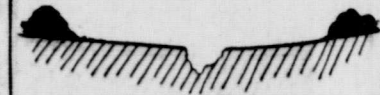
2 Scrape topsoil away from gully. Topsoil is usually bulldozed off to the side into stockpiles.
