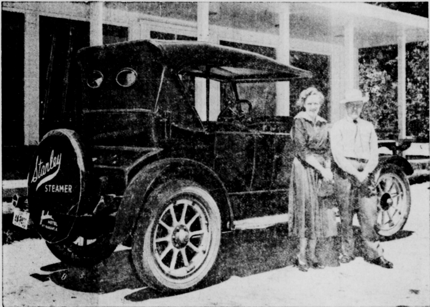
IT'S STILL STEAMIN' ALONG—C. M. McMillan and Ruth Wright stand next to McMillan's 1915-model Stanley Steamer, in Dundee, Ill. The vehicle uses kerosene, gets 12 miles to the gallon and McMillan, from Mt. Pleasant, Ia., was driving it to a county fair.
