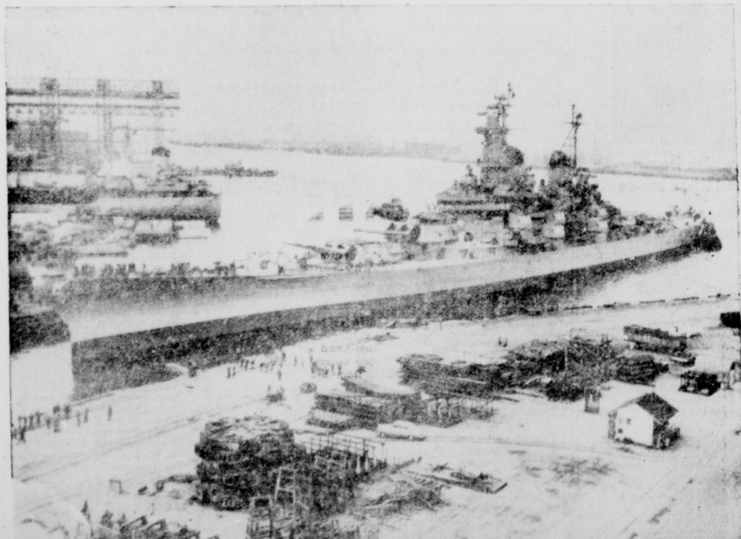
GOING THROUGH TESTS —The battleship Missouri is shown as she goes through dock trials at Norfolk, Va. The trials involve testing the engines which were fouled with mud and sand when the vessel ran aground.
