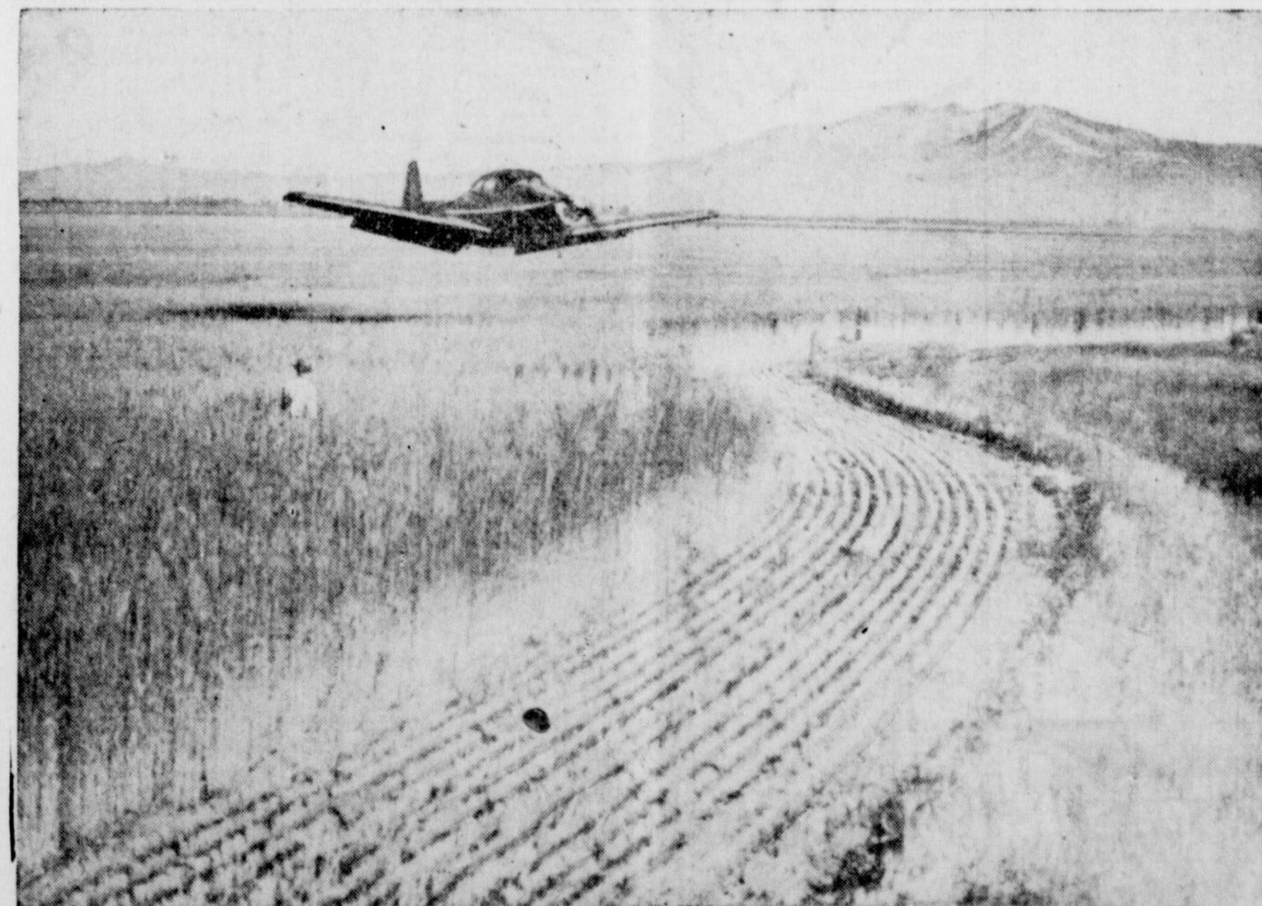
LICKS JACK FROST—One of six Ryan "Navions" makes a pass at a 30-foot altitude over a farm in the Fairfield Valley near Boise, Ida. By churning up the air, planes prevent frost from condensing on the wheat crop below. The experiment, a new application of private planes to ranch work, was successful in preventing frost in the 5000-foot-high valley.
