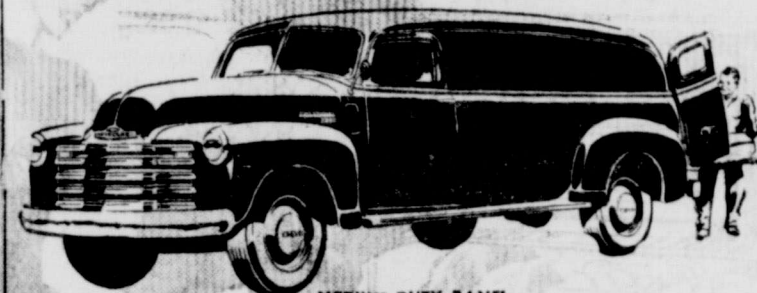
MEDIUM-DUTY PANEL Model 3805—137-inch wheelbase, Maximum G.V.W. 6700 lb. Also available in light-duty Model 3105—116-inch wheelbase, Maximum G.V.W. 4600 lb.
