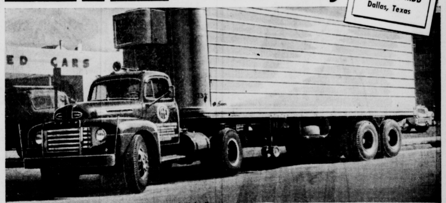
Ford Model F-7 BIG JOB shown has Gross Combination Weight rating of 35,000 lbs. as a tractor; Gross Vehicle Weight rating of 19,000 lbs.
