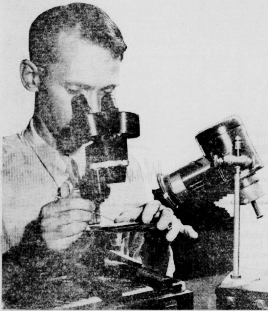
1. Scientists study the tiny shells and other fossils brought up by drillers from the depths of the wells which they are drilling. A close study of these fossils tells them the age of rocks in which the bit is drilling, and enables them to suggest to production men how close they are to possible oil-bearing rocks.
