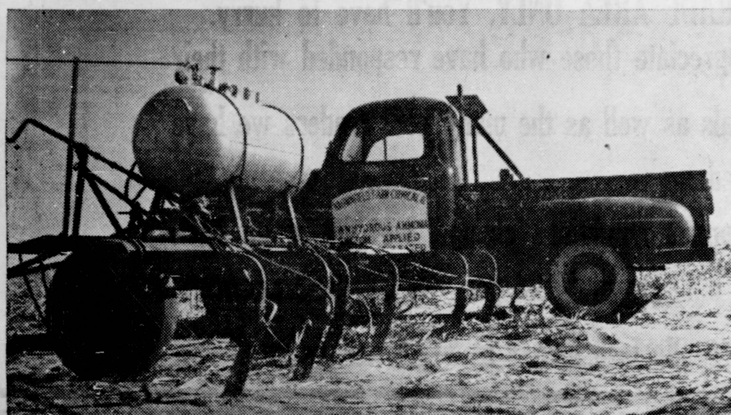
THE DEMPSTER LIQUIJECTOR injects under pressure and chisels the Ammonia deep into the soil where the plant roots will receive full benefit of the application. Agricultural Ammonia will not leach out when injected into the soil. It is virtually independent of weather conditions as it requires no rain to be converted into usable nitrogen.
