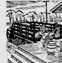
THIS 2-TON CHASSIS is engineered to fit your body needs. On wheelbases of 128", 152", 170", and 192", it will accommodate a wide variety of bodies, from 8 ft. to 181/2 ft. in
