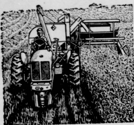
RADDLE TYPE PICKUP—On or off in 15 minutes. For harvesting small grain and seed crops where windrowing is necessary.
