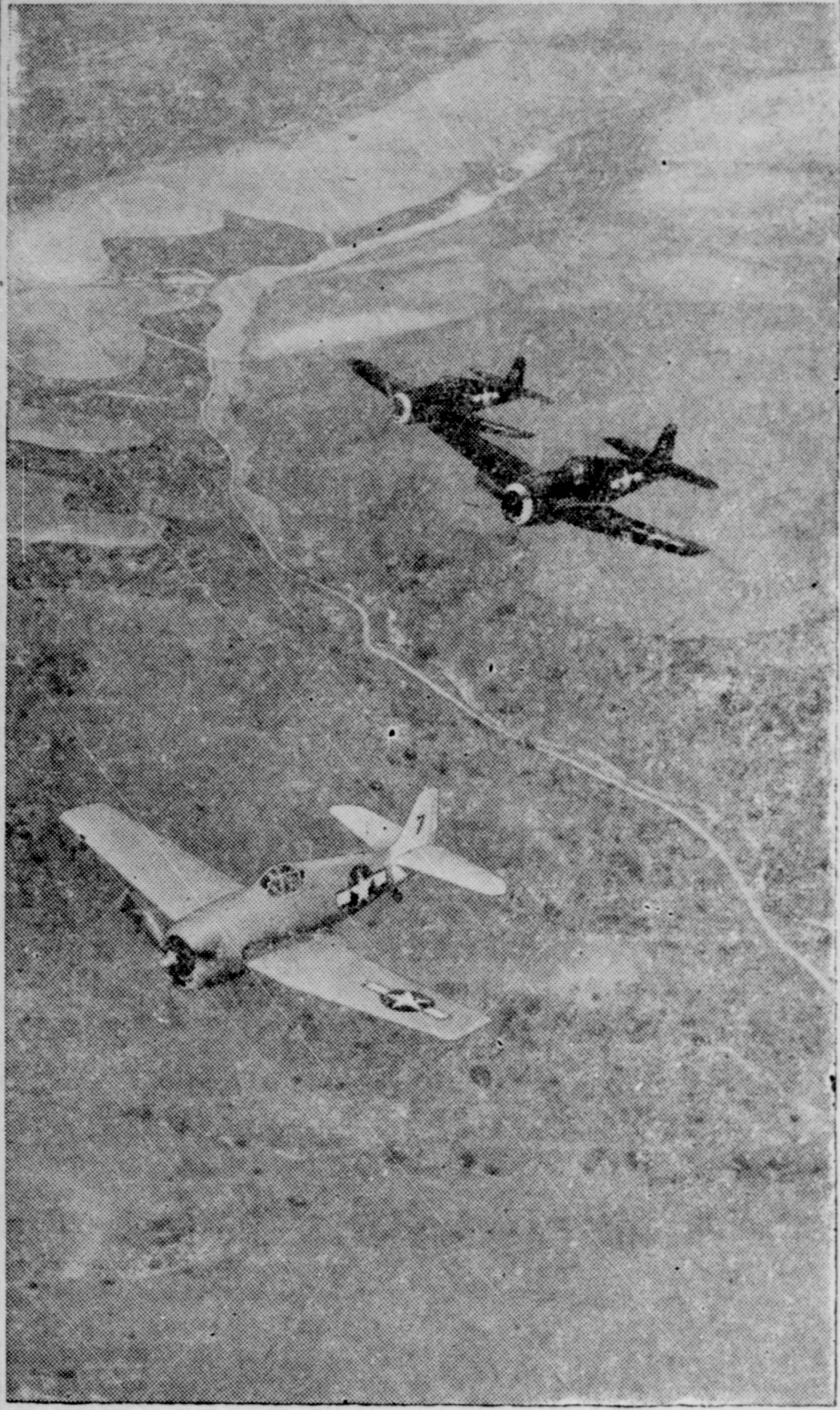
Trailed by two "mother" planes, a pilotless Navy Hellcat (Grumman F6F) soars over the San Diego area in a dress rehearsal for similar air data operations planned as part of the atomic bomb tests at Bikini atoll this summer. The drone (foreground) is controlled by the "mother" Hellcat immediately in the rear while a second plane serves as standby should the first one fail. During the tests four drones, each with two control planes, will be launched from the USS Shangri-la and will be controlled first from the carrier's deck, then from a mother plane in the air and finally from the ground control operator on Roi island where they will land. (Joint Army-Navy Task Force One Photo.)
