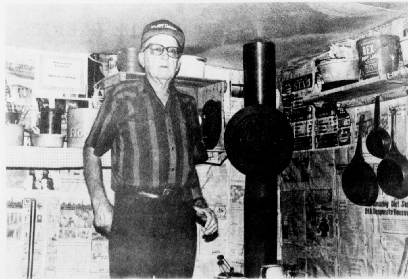
BACHELOR STOVE —A woodburning "Bachelor Stove" is the center workplace for the kitchen corner in the house. An oven is located inside the center of the chimney for baking bread. The kitchen corner is also equipped with cooking wares, Arbuckle coffee, old boxes of baking powder, etc.
