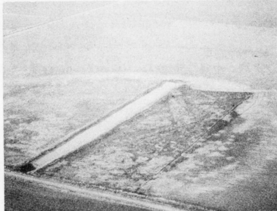
MODIFIED PLAYA LAKE --This aerial photo shows how a modified playa basin collects irrigation water and rainfall runoff in a central location for later re-use. A recent inventory shows approximately 1,289 modified playa basins within the 15 county High Plains Underground Water Conservation District No. 1 service area. Courtesy Photo
