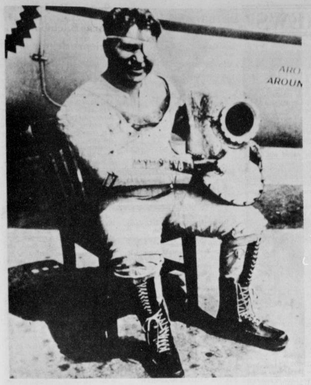
PRESSURE SUIT - Wiley Post dons the final version of his pressure suit. The pressure guage held in his right hand was used to monitor the suit pressure. Just below the left inner knee is seen the outflow port to which the gauge could be attached. Note the ingenious joints at the knee and elbow portions of the suit, facilitating limb motion. The suit was entered at the neck. His Chicago high-altitude flight came on Sept. 4, 1934.
