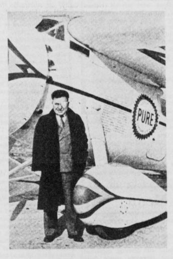
HIGH-ALTITUDE TEST - The "Winnie Mae" in early September 1934, as used in the highaltitude flight-record attempts at Chicago. The sponsoring Pure Oil Company emblem is prominently displayed. The exhaust stacks are separately vented by cylinder and an "external" Bendix supercharged has been added to the top of the Pratt & Whitney Wasp engine. The separate exhaust stacks reduced back pressure and enabled an increase in horsepower, as well as more efficient engine cooling.
