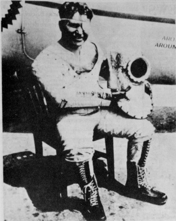
**PRESSURE SUIT** — Wiley Post dons the final version of his pressure suit. The pressure gauge held in his right hand was used to monitor the suit pressure. Just below the left inner knee is seen the outflow port to which the gauge could be attached. Note the ingenious joints at the knee and elbow portions of the suit, facilitating limb motion. The suit was entered at the neck. His Chicago high-altitude flight came on Sept. 4, 1934.
