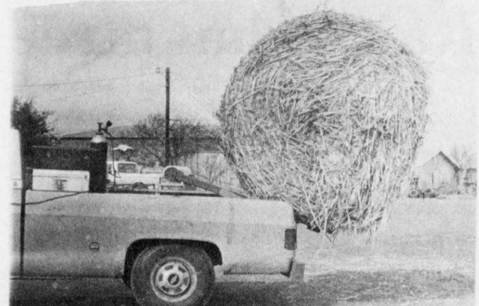
FORTENBERRY'S pick up mounted hay bale loader can be quickly moved from a pick up to a tractor or trailer and loads both round and rectangular bales weighing up to 2250 pounds.
