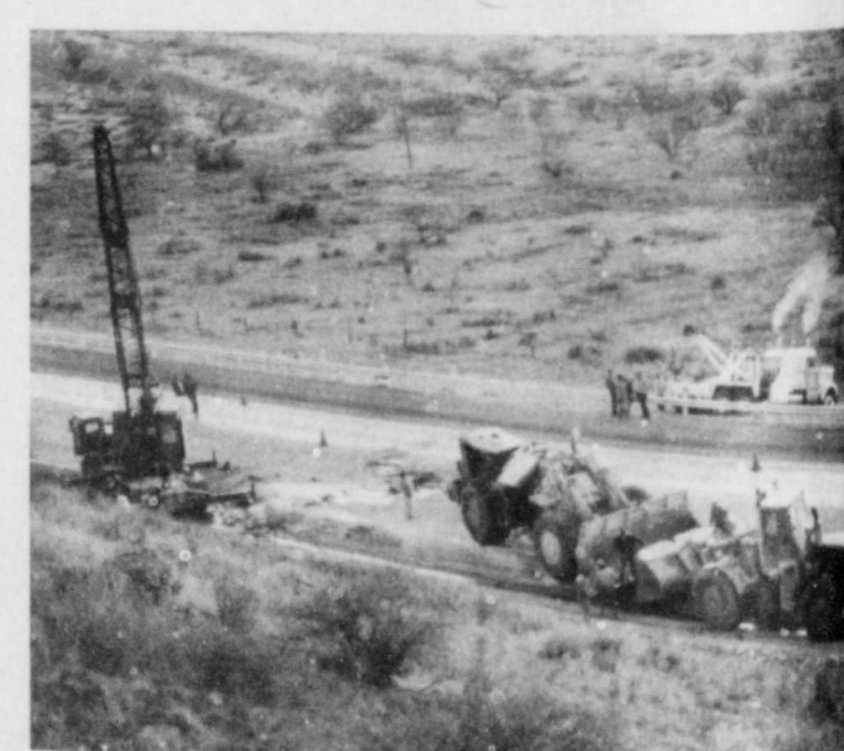
A FRONT END LOADER half the size of the wrecked loader eases the equipment down the hill.
