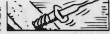
Setting a screw in wood can be made easier if the threads are first coated with soap.
