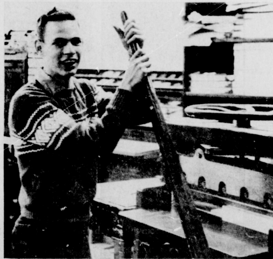
Jimmy Collins cuts just a few of the thousands of sheets of paper that are trimmed each day by this machine.
