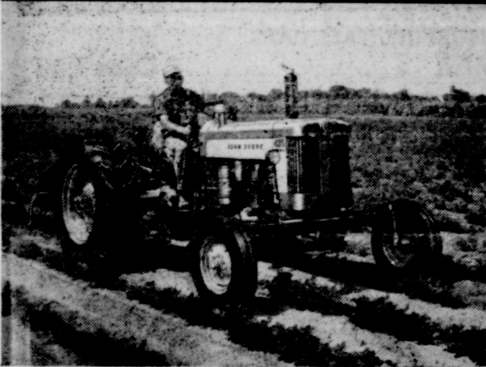
The New John Deere 2-3 plow "435" Diesel Features an ultra-thrifty, electric starting General Motors 2-cylinder, 2-cycle engine—offers new economy and speed!
