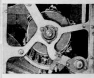
Massey-Harris combines rub the grain out the natural, easy way. The corrugated rasp-bar cylinder - an original Massey-Harris de-velopment - removes the kernels of grain from the straw gently ... yet thoroughly. There are no cylinder teeth to crush the grain. Adjustments can be made quick-ly, easily for the exact speed and clearance best suited for particular crop you're harvesting. The Clipsuccessfully handles more than 110 different grains and grasses.
