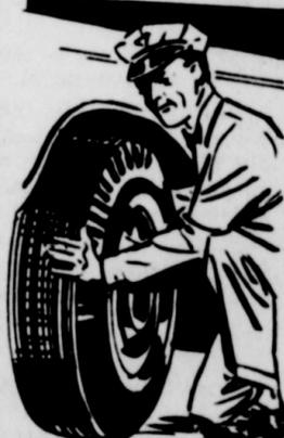
Front tires are subject to wear from steering and braking. Rear tires are worn by the forces of driving, stopping and holding on curves. To equalize this wear and increase tire mileage, tires should be rotated regularly so that they will run in different positions.
