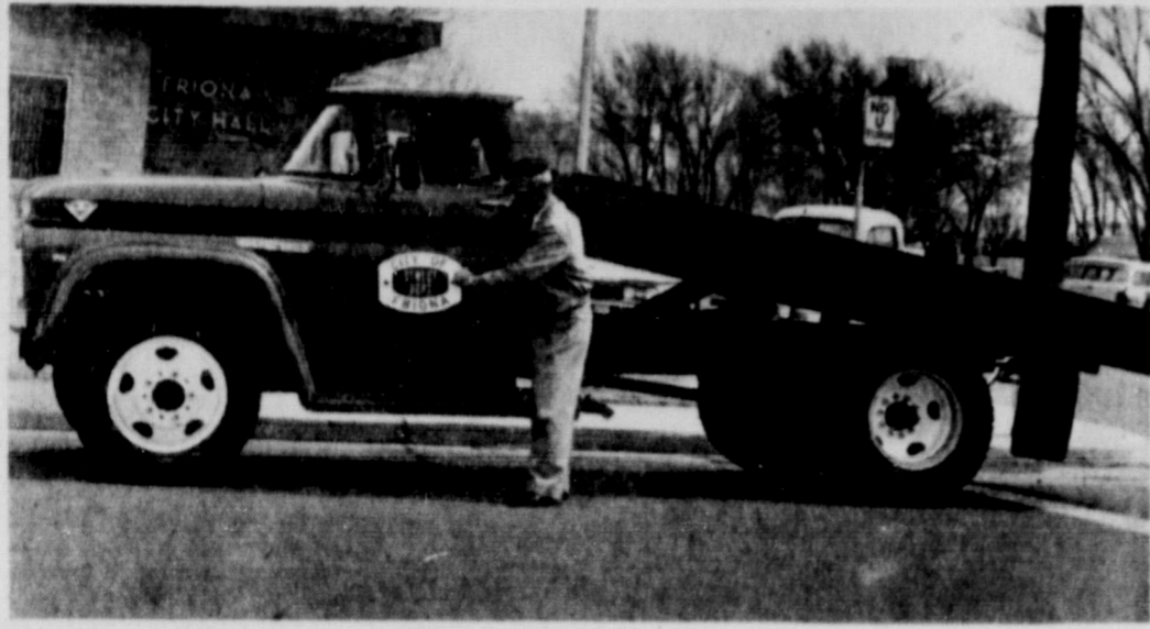
City of Friona decal is being smoothed onto the city's newest piece of equipment by City Manager Jake Outland. The truck, a new GMC, was delivered early this week. It is equipped with a flat bed with a single hoist dump and is to be used for hauling gravel for street repair and for trash collection when necessary.
