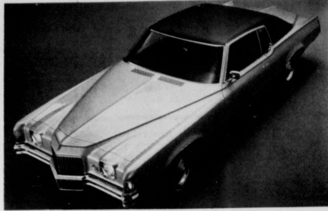
CLASSIC GRAND PRIX -- High-intensity single headlamps, a new vertical bar grille and a two-level bumper highlight the front of the restyled 1971 Grand Prix. The rear has a classic boat tail with new quarter panels, deck lid, bumper and taillights. Standard equipment includes variable ratio power steering, power front disc brakes and a 400 cubic-inch V-8 engine. The SJ package includes a 455 cubic-inch power plant.
