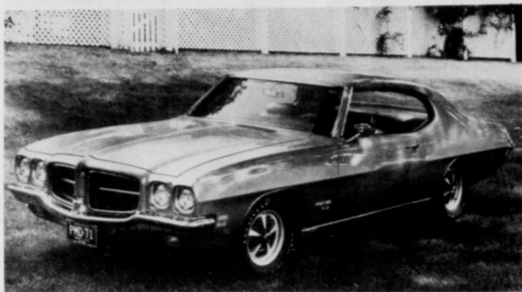
PONTIAC T-37 -- Pontiac Motor Division's 1971 T-37 combines a distinctive appearance with a low price. Standard equipment includes a 250 cubic-inch six-cylinder engine and a manual transmission. Optional are V-8 power plants ranging from 350 to 455 cubic inches and Turbo Hydramatic transmission. The T-37 is available as a two-door hardtop, two-door coupe and four-door sedan.
